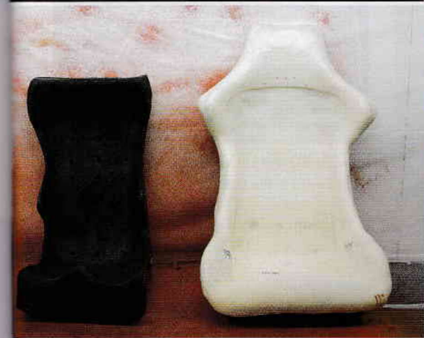
(Top) David Black in Racetech's New Zealand production facility. (Bottom, from right) A custom insert can be added to the standard foam seat pad. The raised ridge in the seat back provides firm mounting to the cage at shoulder level. A Racetech seat installed in a BMW Team RLL Z4 GTE racer.
